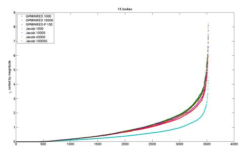
Figure 5. Comparison of solution vector  $\gamma$  for Test Problem 1 (1,000 bodies/3,525 contacts). Here, the solution vector is sorted by magnitude for several methods and different numbers of iterations, corresponding to Table I. Each point is the magnitude of one  $\gamma_i$ .
