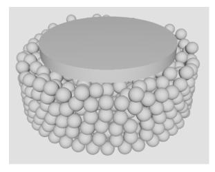
Figure 11. System for Test Problem 3 with 1,001 bodies and  $n_c = 4295$ . The mass of the cylindrical body was set to 1000 kg, 4000 kg, and 16000 kg for the three tests in this set.
