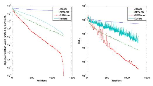
Figure 7. Results for System 2 of Test Problem 2 with  $n_c = 8507$ : Objective function value shifted by a constant and plotted on log axes; Residual  $||\epsilon||_2$  (evaluated as indicated in Eq. (24)).
